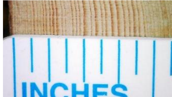
12. At the left, very slow growth rate of about 1/70 inch per year in radius
