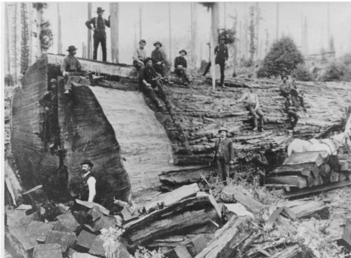
Sawing (“bucking up”) and splitting a huge tree to make railroad ties or other “split product”
