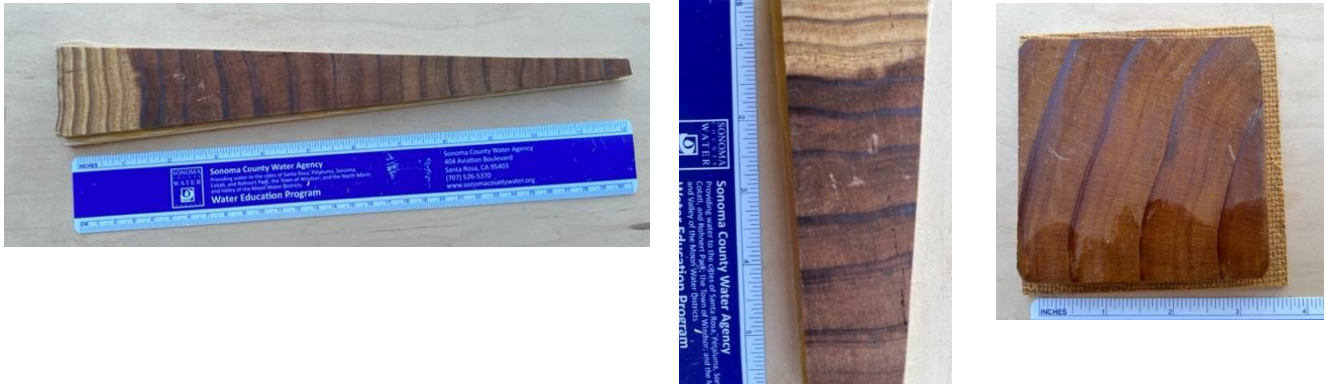
Above left and center: The tree took about 25 years to grow about 12 inches in radius. Above right: section of a 4x4 (3.5"x3.5") fence post. The tree took about 5 years to grow 3.5" in radius.
